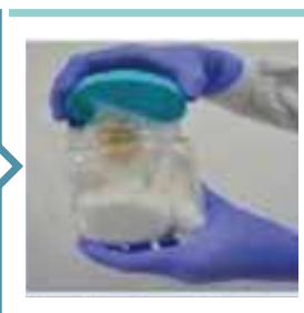
6. Placing the zip - lock pouch inside a study plastic container and seal the neck of the container
